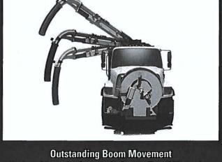
Designed for optimal range, the boom offers 250° rotation, 26' reach, 21' vertical lift and 3' downward pivot to achieve greater work area access and make hose adjustments easier.
