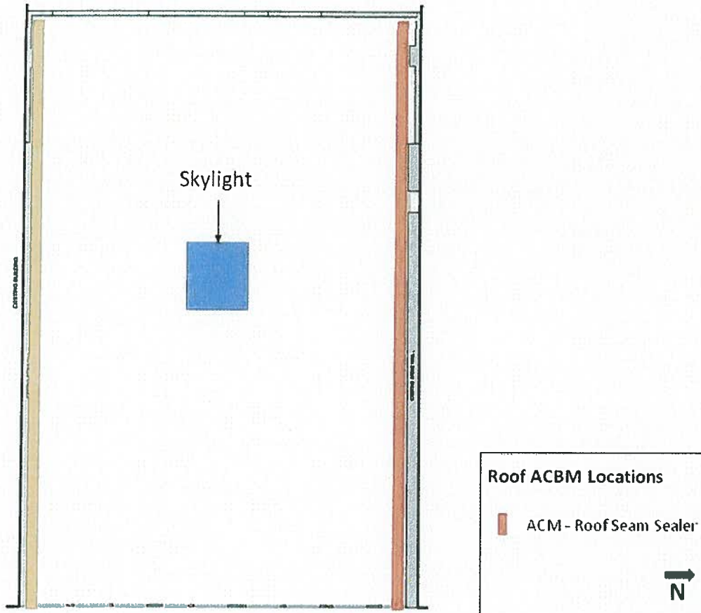
Figure 6. Location ACM roof
